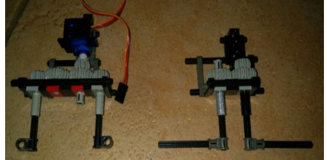
Two Servo motors that allow the movement of both mustaches and eyebrows
