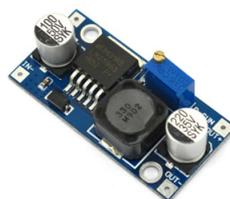
This kind of regulators, with respect to classic linear regulators (e.g. 7805, lm317), let us lower the input voltage to the desired values (acting on a trimmer), yet without having a high heat dissipation that, in a plastic robot, could have led to problems.
