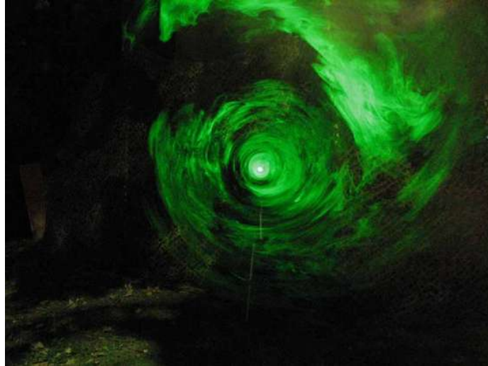
Figure 4.3: Laser vortex example. Created using green laser and rotating mirror.
