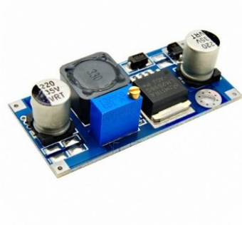
Figure 3.17: LM2596 module. It is a Simple High-Efficiency Step-Down (Buck) regulator.
