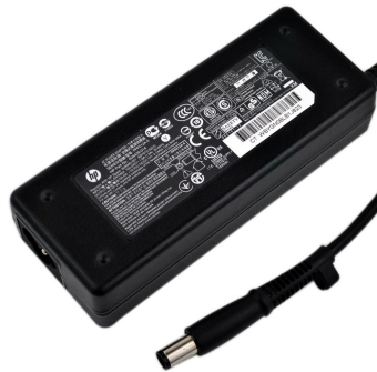
Figure 3.16: Laptop charger used. 65W per 3.5A max.
