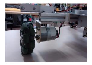
Another problematic part for us was the connection of the motors to the wheels as, by screwing the motor to the metal piece linking the two parts, we broke the metal gear inside the three motors because, as we found out later, we were using too long screws. Since we didn't want to buy new motors, mainly because of the estimated shipping time that would have caused us to lose a week of work on the project, we decided to open them and fix them. Luckily we succeeded by replacing the gears with
